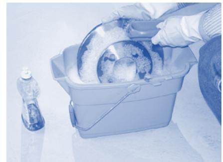
2. Thoroughly clean the calipers, caliper slides and hardware. Remove all dirt, rust and grease.
